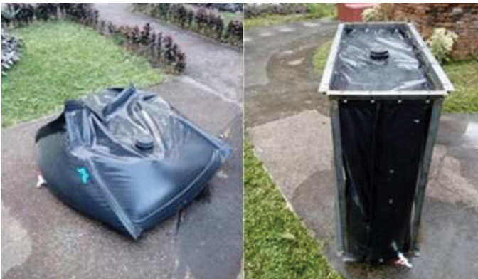
Figure 7. Testing of (a) vertical square-type tank and (b) vertical rectangular type tank
