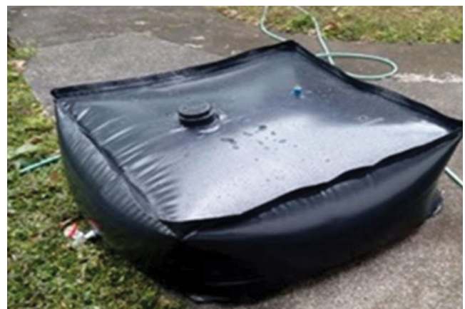
Figure 8. Common types of tanks tested in the site were bladder and square-type CRT
