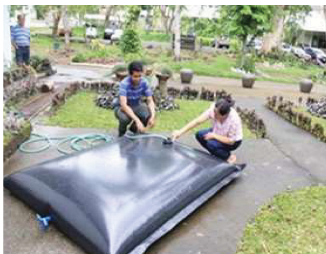
Figure 5. The pillow tank at full capacity
