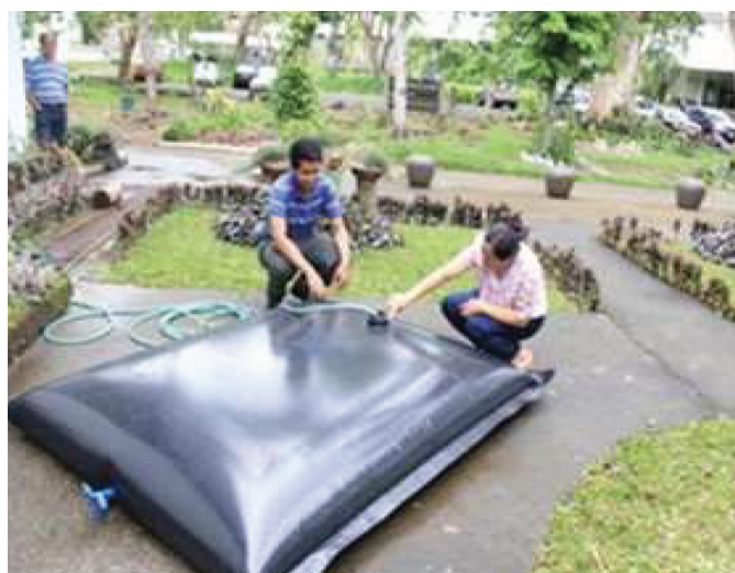
Figure 5. The pillow tank at full capacity
